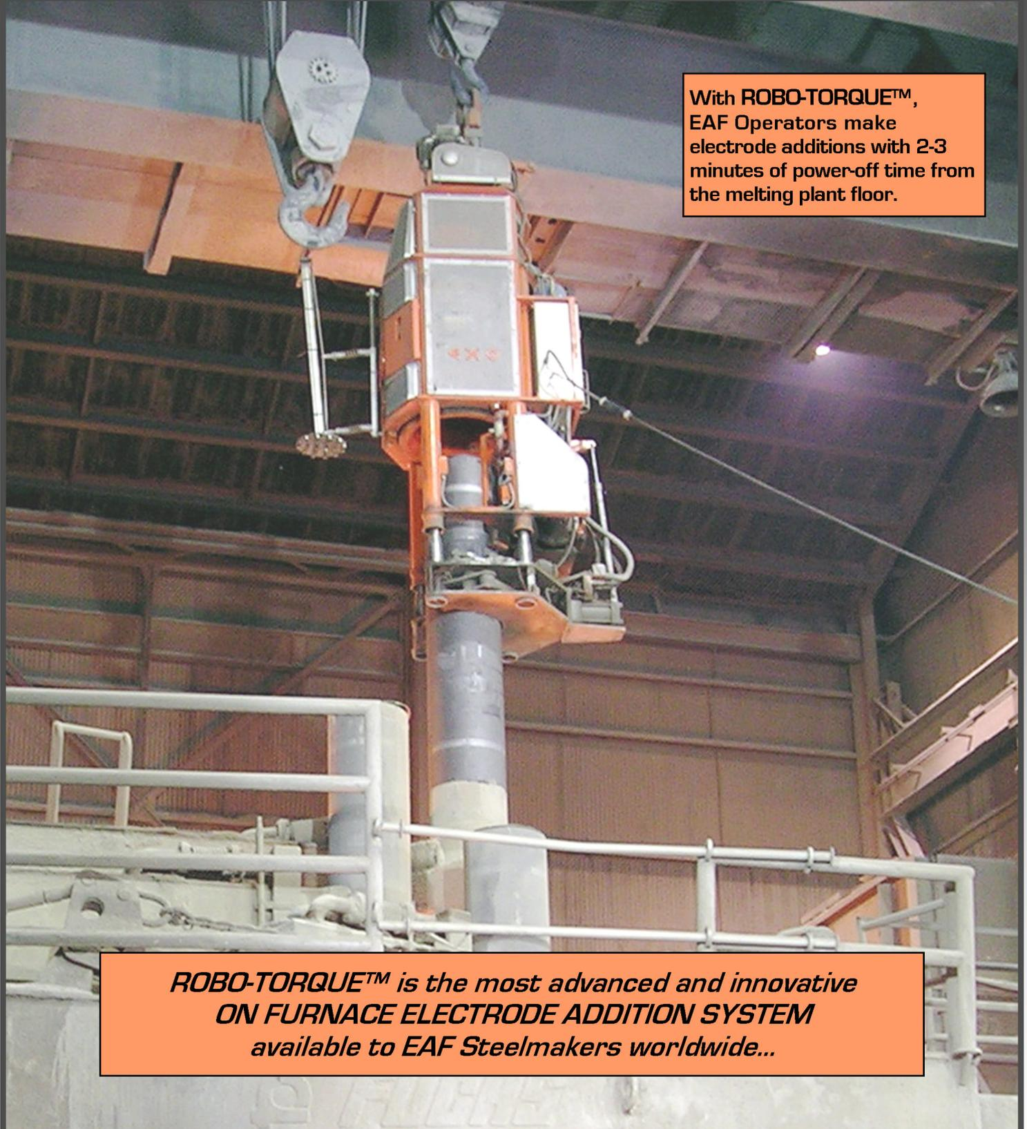
With ROBO-TORQUE™, EAF Operators make electrode additions with 2-3 minutes of power-off time from the melting plant floor.
