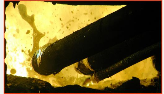
Water-Cooled Supersonic Oxy-Carbon Lance/Burner
