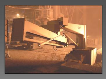
ROBO-TEST™ Auto Steel Test System represents the state-of-the-art in robotic temperature & sampling manipulators. The system automates temperature and chemistry testing in the EAF. Use of the ROBO-TEST™ System reduces accident exposure to Operators, improves accuracy of tests, and reduces delays associated with measurements.
